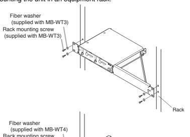
To mount two units in an equipment rack, use the optional MB-WT4 Rack Mount Kit.
